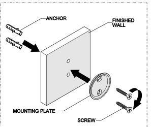
Secure the MOUNTING PLATE onto the finished wall using the SCREWS provided.
