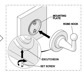
Place the ROBE HOOK over the MOUNTING PLATE then thread and securely tighten the SET SCREW into the ESCUTCHEON.
