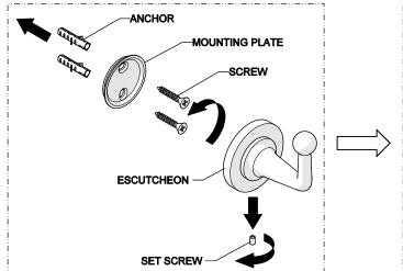
Unthread the SET SCREW and remove the MOUNTING PLATE, SCREWS and ANCHORS from ROBE HOOK.
