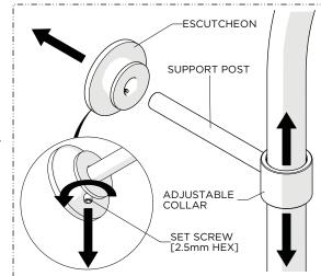
Loosen, but do NOT remove, the SET SCREW using a 2.5mm HEX KEY to remove the SUPPORT ESCUTCHEON from the SUPPORT POST then, if necessary, adjust the height of the COLLAR.
