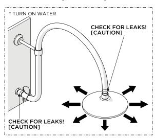
Turn on the water and operate the SHOWER HEAD to ensure it pivots and functions properly. Inspect all connections for leaks then turn the water off.
