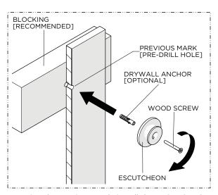
Using the previous mark, install the ESCUTCHEON using the WOOD SCREW provided.
