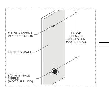
Mark the location for the SUPPORT POST from the center of the NIPPLE to the desired on-center spread.
