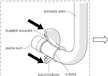
Slide the INLET ESCUTCHEON and RUBBER WASHER up the SHOWER ARM to expose the UNION NUT.
