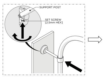
7. Making sure the SUPPORT POST is fully inserted into the ESCUTCHEON, thread and securely tighten the SET SCREW.
