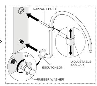
Align the NUT to the NIPPLE and the POST to the ESCUTCHEON then thread and securely tighten the NUT onto the NIPPLE making sure the POST fits properly into the ESCUTCHEON.
