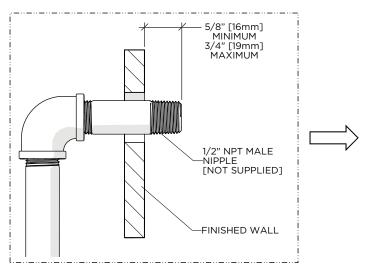
Ensure the front face of the 1/2" NPT MALE NIPPLE (not supplied) is 5/8" [16mm] to 3/4" [19mm] in front of the finished wall.
