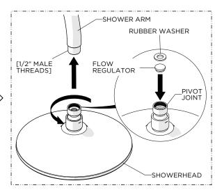
Insert the RUBBER WASHER into the PIVOT JOINT on the SHOWER HEAD then thread and securely tighten the PIVOT JOINT onto the SHOWERARM.
