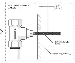
Mark the VOLUME CONTROL CARTRIDGE STEM 5/8" [16mm] beyond where it protrudes from the finished wall.
