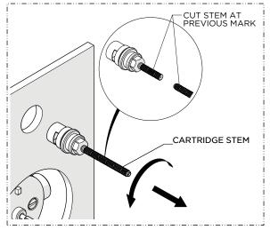
7. Remove the VOLUME CONTROL CARTRIDGE using a 21/32" [17mm] shower valve socket wrench (not provided) then cut the STEM at the previous mark.
