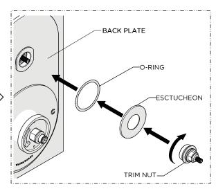
11. Hold the ESCUTCHEON against the BACK PLATE and thread the TRIM NUT into the TRIM CONNECTOR and securely tighten using a 5/8" [16mm] wrench.
