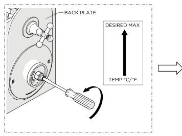
19. With water running, rotate the SQUARE TUBE to adjust the temperature to the maximum desired bathing temperature, verified with a thermometer. Turn the water off and make sure not to change this setting.
