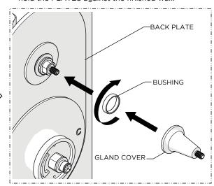
12. Thread the PLASTIC BUSHING onto the TRIM NUT then place the GLAND COVER onto the TRIM NUT making sure it is fully seated.
