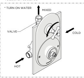
17. Turn on the water supply and open the VOLUME CONTROL VALVE to run water through the THERMOSTATIC VALVE.
