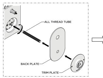
Thread the ALL THREAD TUBE onto the THERMOSTATIC CARTRIDGE then slide the BACK PLATE and TRIM PLAET over the TUBE.
