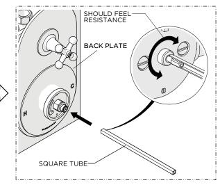
14. Insert the SQUARE TUBE into the TRIM NUT then, by feel, make sure it slides over the CARTRIDGE STEM and is fully seated.
