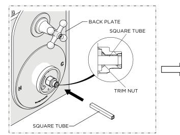
16. Re-insert the SQUARE TUBE back into the TRIM NUT making sure it is slight recessed.
