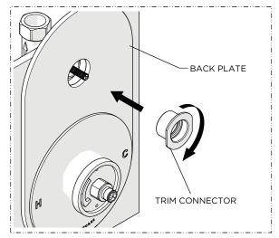
Thread and securely tighten the TRIM CONNECTOR onto the THREADED TUBE.
