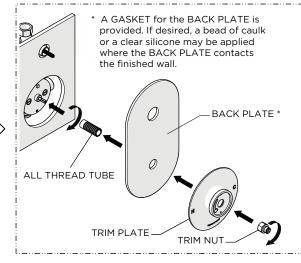
9. Thread the ALL THREAD TUBE back onto the THERMOSTATIC CARTRIDGE, slide the BACK and TRIM PLATES over the TUBE then thread and securely tighten the TRIM NUT onto the TUBE to hold the PLATES against the finished wall.
