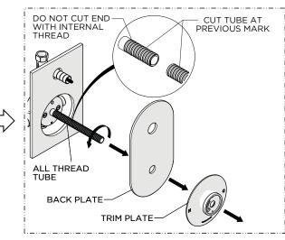
Remove the TRIM PLATE, BACK PLATE and TUBE then cut the TUBE at the previous mark. Do NOT cut the end with internal threads.
