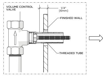
4. Mark the THREADED TUBE 1/4" [6mm] behind the finished wall.
