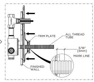
2. Firmly holding the PLATES against the wall, mark the TUBE 3/16" [5mm] beyond where it protrudes from the TRIM PLATE.
