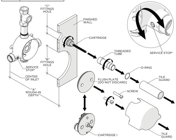
IMPORTANT: The CARTRIDGE is packaged separately and provided with the VALVE.
