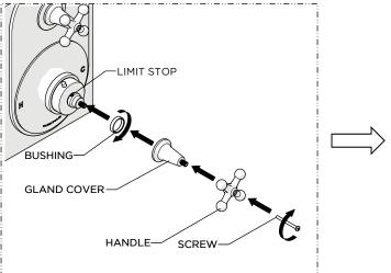
23. Thread the BUSHING back onto the LIMIT STOP, place the GLAND COVER onto the LIMIT STOP and over the BUSHING, place the HANDLE onto the GLAND COVER in the desired orientation, then thread and securely tighten the SCREW.
