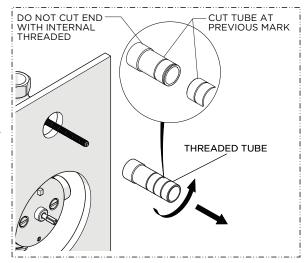
Unthread the THREADED TUBE then cut the TUBE at the previous mark. Do NOT cut the end with the internal thread.
