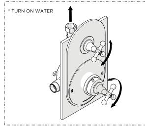
24. Turn on the water supply and operate the HANDLE to ensure that it is functioning properly.
