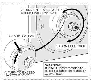
22. Turn the LIMIT STOP to cold then hot and confirm it is functioning properly. Verify the maximum desired bathing temperature. To get a hotter temperature, press and hold the LIMIT STOP BUTTON and turn the LIMIT STOP further.
