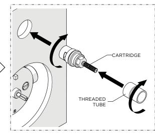
8. Thread and securely tighten the CARTRIDGE back into the VOUME CONTROL VALVE then thread the TUBE back onto the CARTRIDGE.
