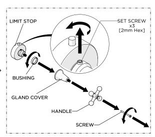
20. Unthread the SCREW, remove the HANDLE, remove the GLAND COVER, and unthread the BUSHING to expose the SET SCREWS then loosen the SET SCREWS using a 2mm hex key.
