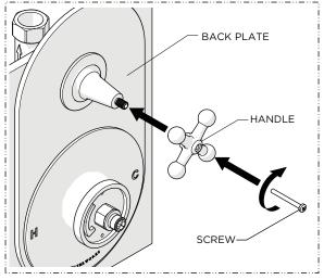
Place the HANDLE onto the GLAND COVER in the desired orientation then thread and securely tighten the SCREW.
