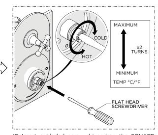
18. Insert a bladed screw driver into the SQUARE TUBE. Slowly rotate the TUBE clockwise to attain full cold then counterclockwise to attain full hot. It's approximately 2 complete rotations. Verify a full range of temperatures exists.
