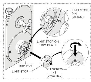
Place the LIMIT STOP over the TRIM NUT making sure the LIMIT STOP PIN makes contact with the LIMIT STOP on the TRIM PLATE then tighten the SET SCREWS.
