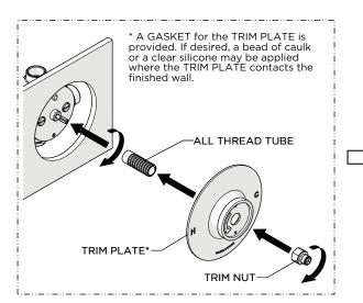
4. Thread the TUBE back onto the CARTRIDGE, slide the PLATE over the TUBE, and thread the TRIM NUT onto the TUBE. Securely tighten to hold the PLATE against the finished wall. SHOULD FEEL
