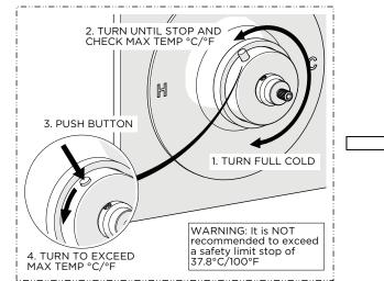
13. Turn the LIMIT STOP to cold then hot and confirm it is functioning properly. Verify the maximum desired bathing temperature. To get a hotter temperature, press and hold the LIMIT STOP BUTTON and turn the LIMIT STOP further.
