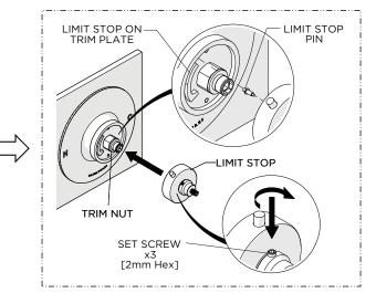
12. Place the LIMIT STOP over the TRIM NUT making sure the LIMIT STOP PIN makes contact with the LIMIT STOP on the TRIM PLATE then tighten the SET SCREWS.
