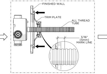
2. Firmly holding the PLATE against the finished wall, mark the TUBE 3/16" [5mm] beyond where it protrude from the PLATE.
