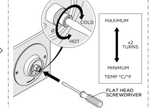
9. Insert a bladed screw driver into the SQUARE TUBE. Slowly rotate the TUBE clockwise to attain full cold then counterclockwise to attain full hot. It's approximately 2 complete rotations. Verify a full range of temperatures exists.
