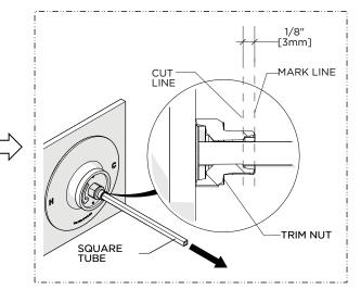
6. Mark the SQUARE TUBE where it passes through the front face of the TRIM NUT then remove and cut the TUBE 1/8" [3mm] behind the previous mark.
