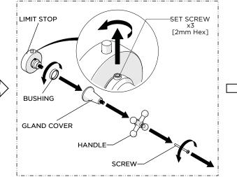
Unthread the SCREW, remove the HANDLE, remove the GLAND COVER, and unthread the BUSHING to expose the SET SCREWS then loosen the SET SCREWS using a 2mm hex key.
