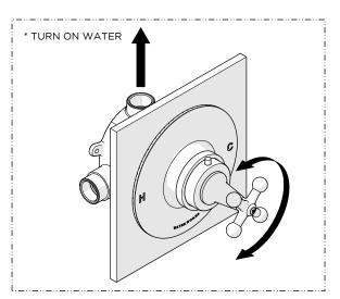
15. Turn on the water supply and operate the HANDLE to ensure that it is functioning properly.
