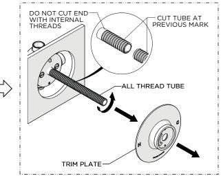
3. Remove the TRIM PLATE and ALL THREAD TUBE, then cut the TUBE at the previous mark. Do NOT cut the end with the internal threads.
