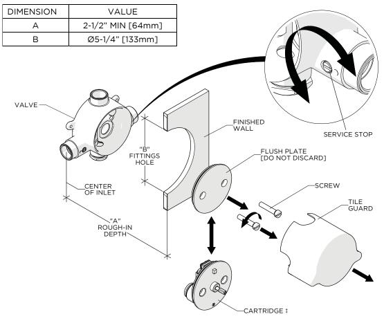
‡ **IMPORTANT:** The CARTRIDGE is packaged separately and provided with the VAVLVE.
