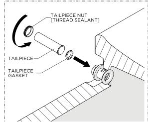
Attach the TAILPIECE to the DRAIN FLANGE using the GASKET and NUT; a thread sealant is recommended and may be applied to the FLANGE threads.
