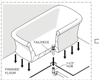
10. Move the BATHTUB into position and align the TAILPIECE with the HUB then carefully lower the BATHTUB until it fully rests on the finished floor.
