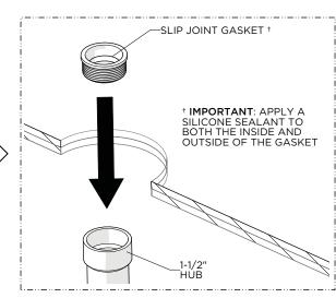
Apply a generous coating of silicone sealant to both the inside and outside of the SLIP JOINT GASKET and insert the GASKET into the HUB.
