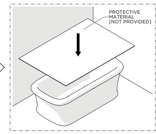
15. Cover the BATHTUB surface with a liner or other protective material (not provided) until construction is completed.
