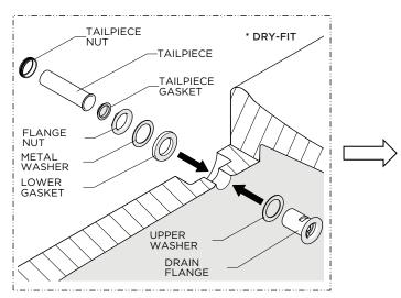
4. Cover the floor with a pad or other protective material and gently rest the BATHTUB on its side then dry-fit the DRAIN (PTWO04 is shown - SOLD SEPARATELY).
