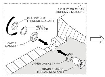
7. Apply a generous amount of putty or a bead of a clear adhesive silicone to the UPPER and LOWER GASKETS and set the FLANGE. Thread and securely tighten the NUT; a thread sealant is recommended and may be applied to the FLANGE threads.
