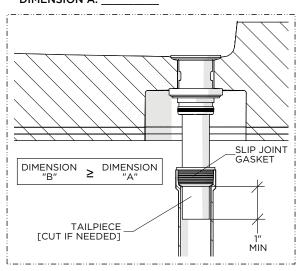
6. IMPORTANT: Verify DIMENSION B is greater than or equal to DIMENSION A. This will ensure that the TAILPIECE will extend a MINIMUM of 1" past the SLIP JOINT GASKET. If necessary, cut the TAILPIECE.
