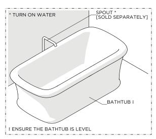
Verify the BATHTUB is level and, if needed, add shims then fill the BATHTUB until water enters the overflow hole.
