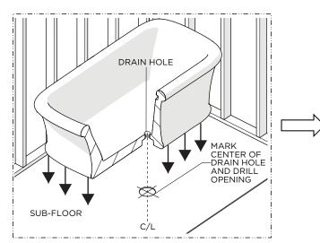
1. Determine the placement of the BATHTUB and mark the location of the drain hole then drill a hole through the floor to accommodate the DRAIN (sold separately).
