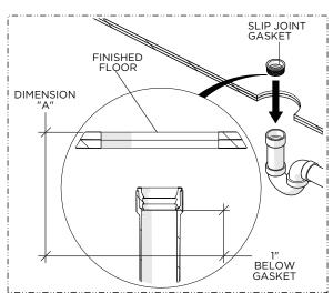
3. Insert the SLIP JOINT GASKET into the HUB then measure from the finished floor to 1" past the bottom of the GASKET.
