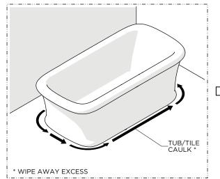
14. Run a bead of tub and tile caulk around the bottom edge of the BATHTUB where it meets the finished floor; wipe away any excess caulk with a wet paper towel
