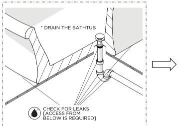
13. Drain the BATHTUB and inspecting all connections above and below the finished floor for leaks.
