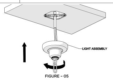
14. Thread the LIGHT ASSEMBLY to the NIPPLE on the MOUNTING PLATE making sure it's secure.
