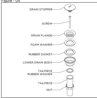
16. Set the drain flange in the lavatory drain opening using putty or a clear adhesive silicone depending on the mounting surface material.\* Re-install the lower drain body with the screw, making sure to use the rubber gasket provided and tighten until fully secured. Putty or a clear adhesive silicone may be used to ensure a water-tight seal between the gasket and lavatory.\* See Figure - 06.
