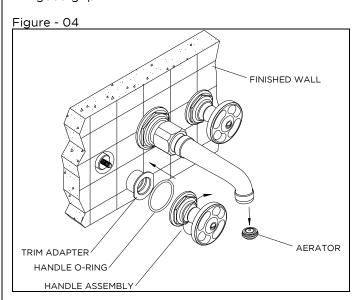
These guidelines have been prepared for the professional contractor to aid in the installation of: RWATLAS WALL MOUNTED LAVATORY WITH METAL WHEEL HANDLES (STYLE# RWLS60) & METAL LEVER HANDLES (STYLE # RWLS70)
