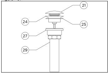
Set the drain flange (24) in the lavatory drain opening using putty or a clear adhesive silicone depending on the mounting surface material.\* Reinstall the lower drain body (27) making sure to use the rubber gasket (26) provided and tighten until fully secured. Putty or a clear adhesive silicone may be used to ensure a water-tight seal between the gasket and lavatory.\*
