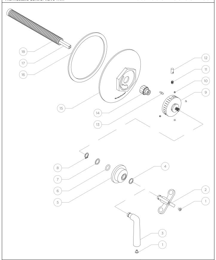
These guidelines have been prepared for the professional contractor to aid in the installation of: HENRY THERMOSTATIC CONTROL VALVE TRIM METAL CROSS HANDLE (HNSV01) AND METAL LEVER HANDLES (HNSV10).
