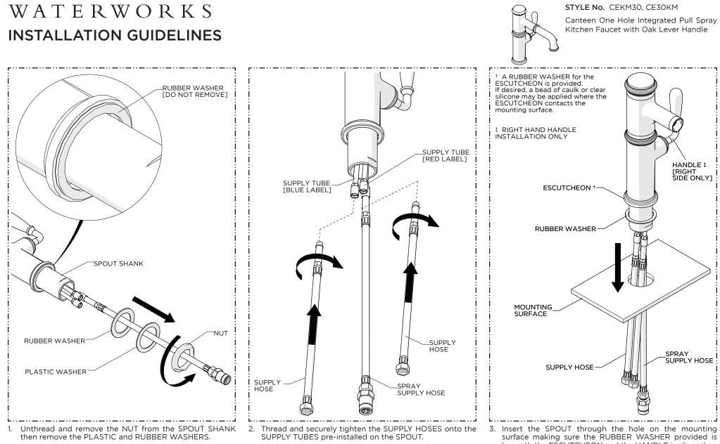
NOTE: Do NOT remove the RUBBER WASHER beneath the ESCUTCHEON.
