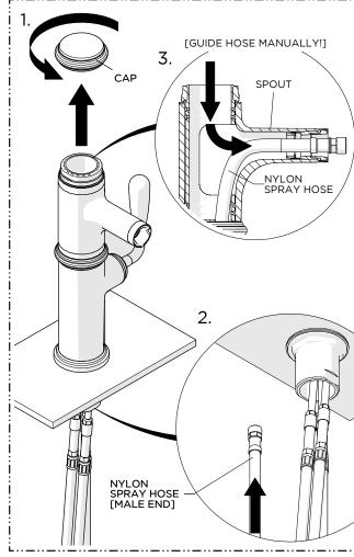
Unthread and remove the CAP from the top of the SPOUT then insert the MALE END of the NYLON SPRAY HOSE through the bottom of the SPOUT and, from above, manually guide the HOSE out of the SPOUT.
