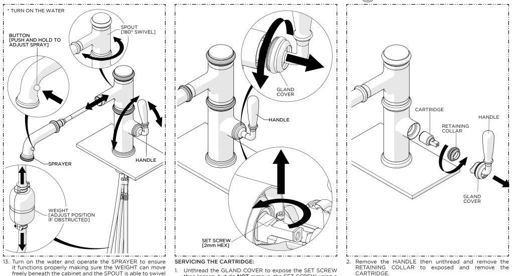
properly. Adjust the position of the WEIGHT if necessary.
