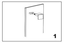
Install the Knob-A (bolt) through the glass hole, make sure the rubber gaskets are between knob&glass.
