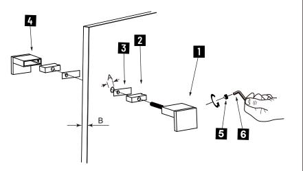
1.Knob-A x 1 2.Fixing Bracket x 2 3.Clear Gasket x 2 4.Knob-B x 1 5.Set Screw M5 x 1 6.Allen Key 2.5mm x 1
