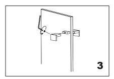
Add the knob-B end on the fixing bracket.
