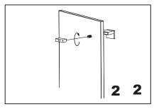
Fix the fixing bracket onto the knob A bolt.
