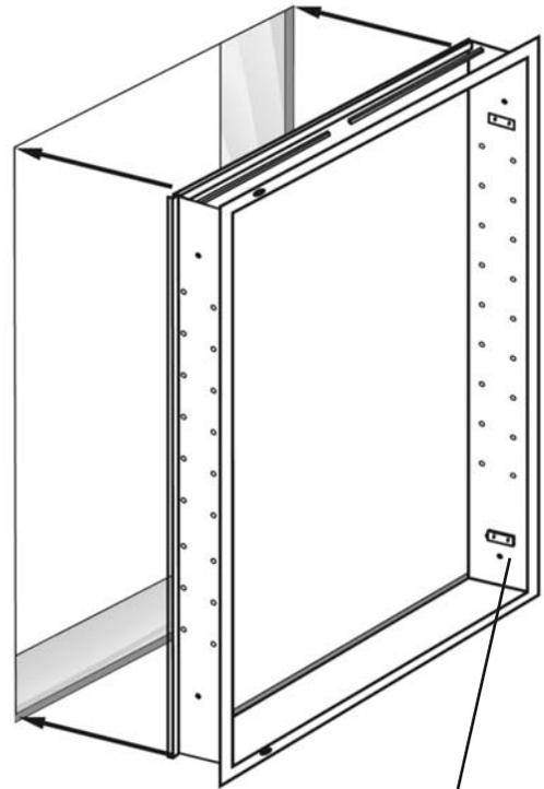
Hinge Plate shown for right hinged door. Handed door is determined at the time of order. Be sure to install with left or right hinged unit on the correct side.
