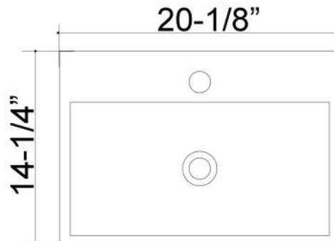
Dimensions of fixture are nominal and may vary within the range of tolerances established by ASME Standard A112.19.2.2013 Dimensions and specifications subject to change without notice.
