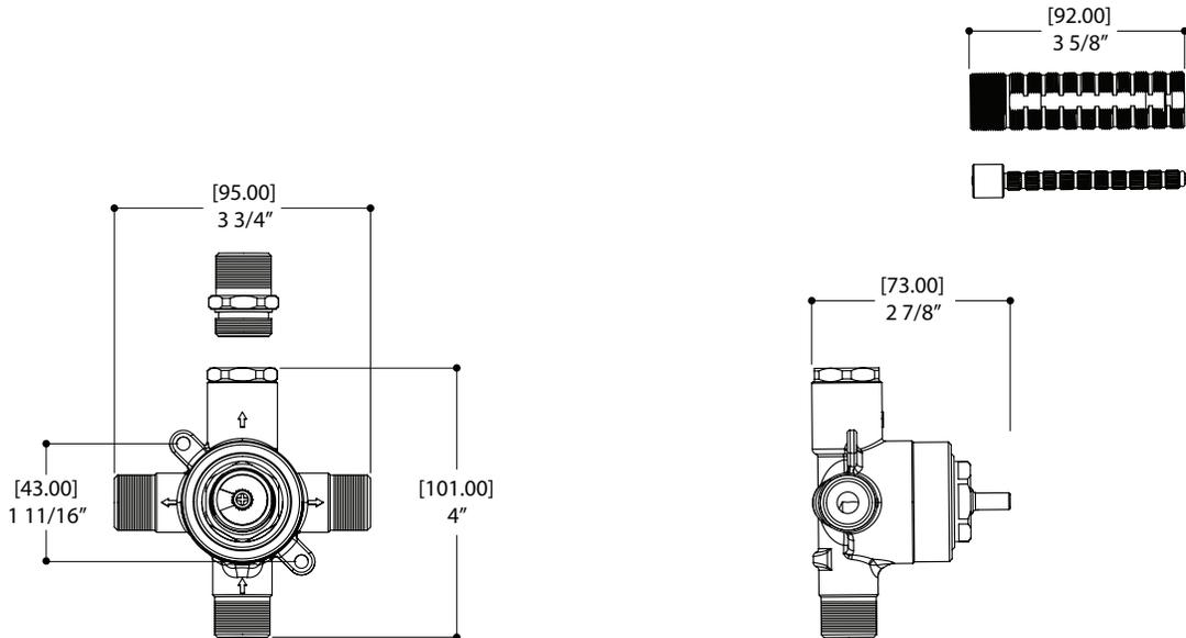
Turbo totem T12000 - 3/4" - 1/2" Thermostatic valve - Valve thermostatique 3/4" - 1/2"
